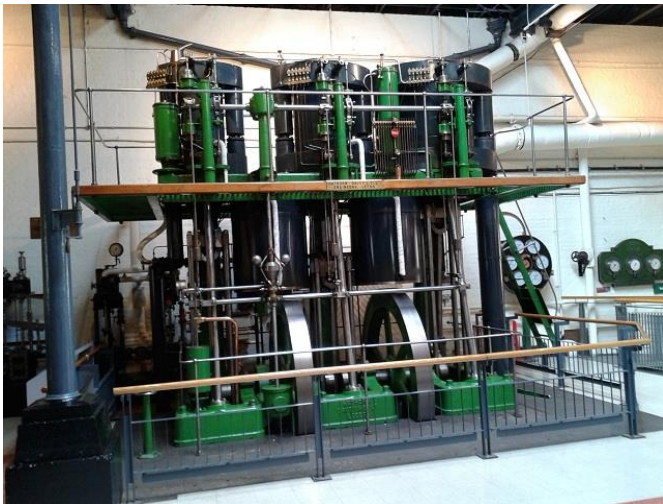
Vertical triple expansion engine, Hathorn Davey, Leeds
