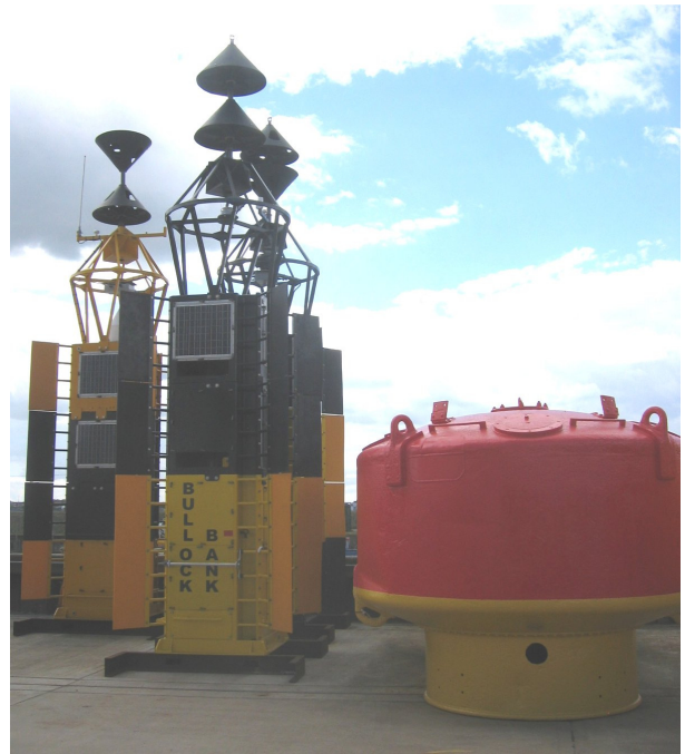
Type 1 Buoy showing buoyancy tank and superstructure
