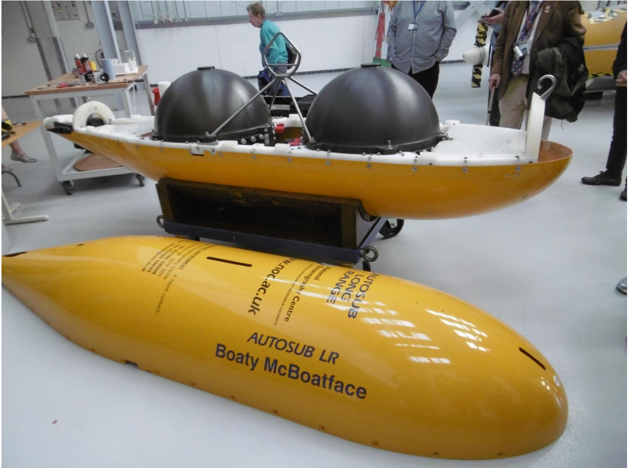
One sphere is for the batteries and the other electronics. Completely automated.
